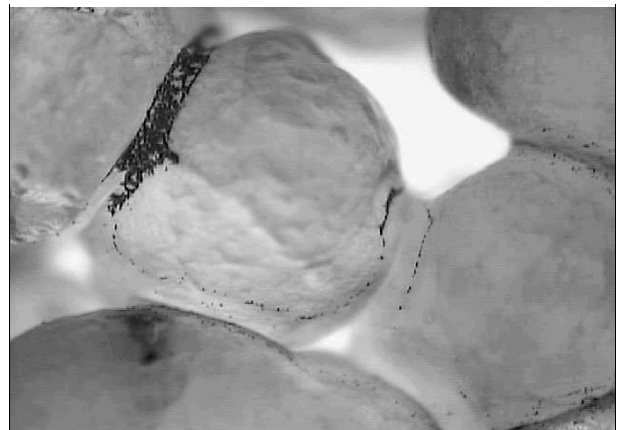
Figure 5: Coagulant hydrophilic colloids formed "bridges" between the grains.
